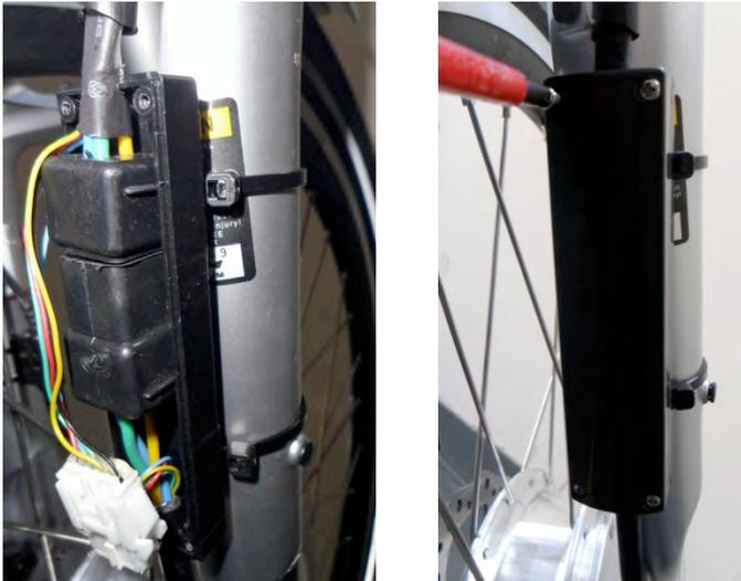
Attach motor cable junction box cover to the front fork, push connectors together and close the junction box with the self tapping screws provided. Be careful to place wires carefully so that they do get pinched by the cover.
