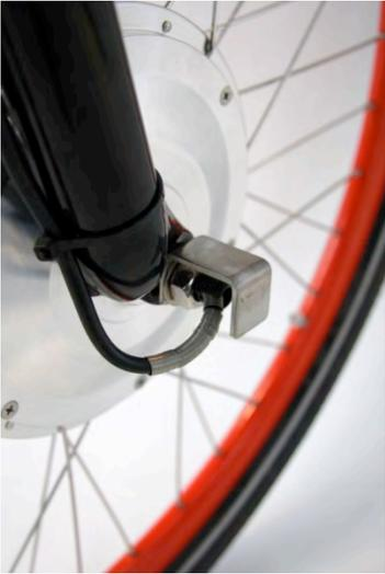
Front wheel with cable protection bracket
