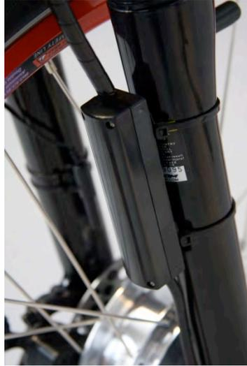
Junction box cover for motor cable connectors
