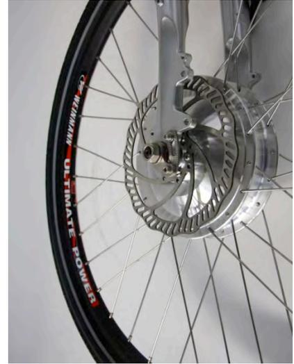
Front wheel left side with disc brake rotor and universal torque plates
